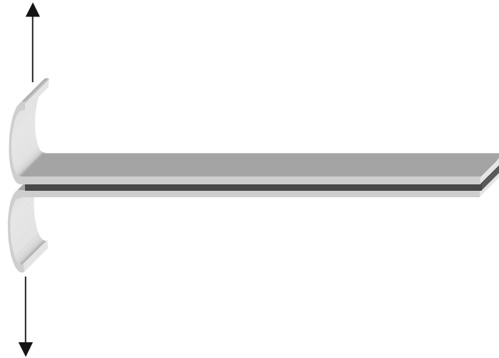
FIGURE 27.2. Diagram of an ASTM D1876 T-peel specimen.
