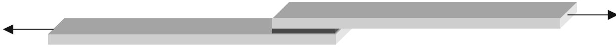
FIGURE 27.1. Diagram of an ASTM D1002 lap shear specimen. The adherends are usually 2.54 cm wide and 10.16 cm long. The thickness of the adherend depends upon the adherend material. If the adherend is aluminum, that thickness is usually 0.16 cm thick.
