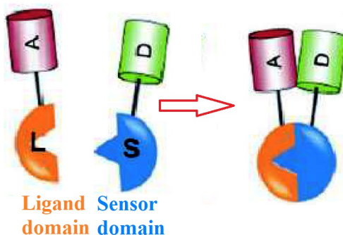
Fig. 3. A nano-sensor that produced FRET signals was developed to identify Kras oncogene point mutations in ovarian tumors [reprinted from ref. 15 with permission].
